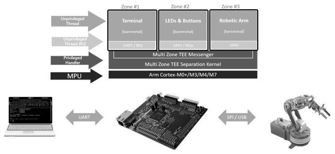
Fig. 3 - Multi Zone Trusted Execution Environment - Reference Implementation Architecture.
